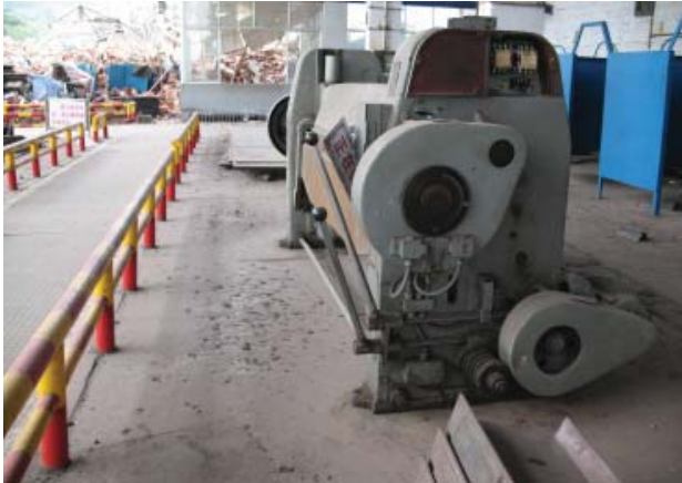
Figure 25. Sliding of Non-Anchored Equipment
